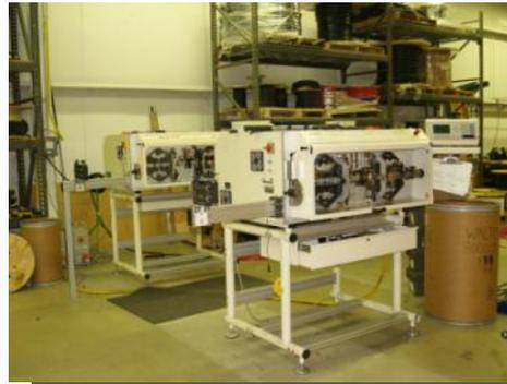
These semi-custom cut and strip machines can process cable from 8 awg (12mm) - 252 MCM (37mm). They can also process multi-conductor cable up to 325 feet long from 6.5 inches at a
