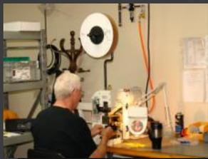
Our Molex crimpers TM-4000 (shown) and TM-3000 give us a superior and accurate crimp. The TM-4000 is a 4.7 ton press used for insulated and non-insulated terminals up to 2awg. This is one of our most versatile machines. The TM-3000 is a 2.7 ton press that offers similar results just at smaller wire sizes.
